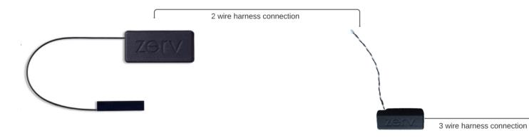
Only the positive and negative leads of the zerver b 6-wire harness are used in this solution. The Data1/Data 0 wires of the 6 wire harness are not used.
