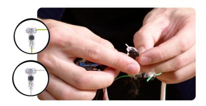
**5** Splice the IDC of the red Zerver B conductor inline with the red(+) conductor of the reader wiring harness. Do **NOT** cut the wire on either side of the IDC Splice.
