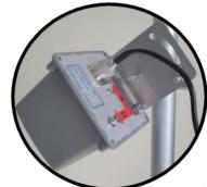
Strain relief the BT cable by bending it along the side of the Zerver B and then wrapping a piece of electrical tape around it as shown below.
