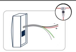
**6** Repeat Step 5 - splicing the black conductors of the Zerver B and reader wiring harness together. Remember to use Pliers to securely clamp the IDCs.
