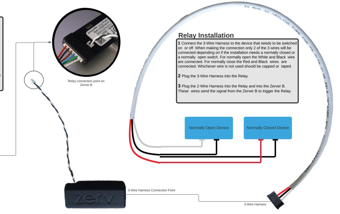
**Relay Wiring Guide W/O control panel (Inteligent Readers)**
