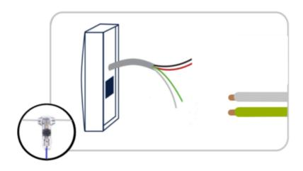
**2** Repeat **Step 1** - connecting the brown conductor from the Zerver B harness to the green Data1 conductor from the reader harness.
