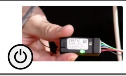
**8** When re-installing the reader with a Zerver B attached: remove the bottom or lower side knockout from reader gang box to allow routing of the LoRa antenna to the outside of the box.
