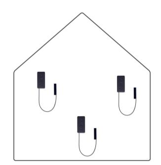
To utilize the data-logging and remote device management capabilities of the Zerver B, a LoRa network will need to be implemented. The LoRa Network consists of A single MultiTech gateway that covers up to 2 miles range with minimal obstruction. The gateway is connected to the specified network via ethernet or wireless SIM card based 4G LTE wireless provider.
