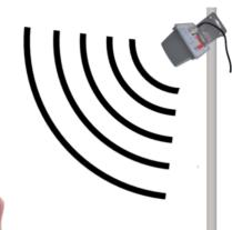
Attach the RP-SMA connector to the RP-SMA to N-Type Cable Assembly. The Zerver B needs to be mounted inside the cabinet to protect it from the environmental elements. The cable then runs out of the cabinet to the externally mounted Directional BT Antenna. The N-Type connector screws into the back of the Directional BT Antenna. The antenna should be low and pointed down at where the car will be. It can be pole mounted as shown below.
