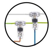
**3** To place the Zerver B between the reader and control panel, cut the white/Data0 and green Data1 condcutors on the control panel side of the IDC.
